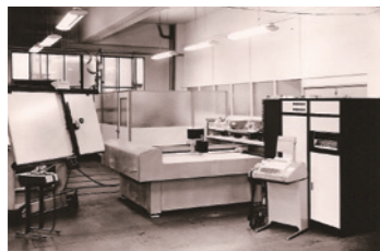
Grading machine modifies and cuts basic sewing patterns to match each size
