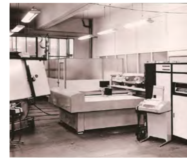
Grading machine modifies and cuts basic sewing patterns
